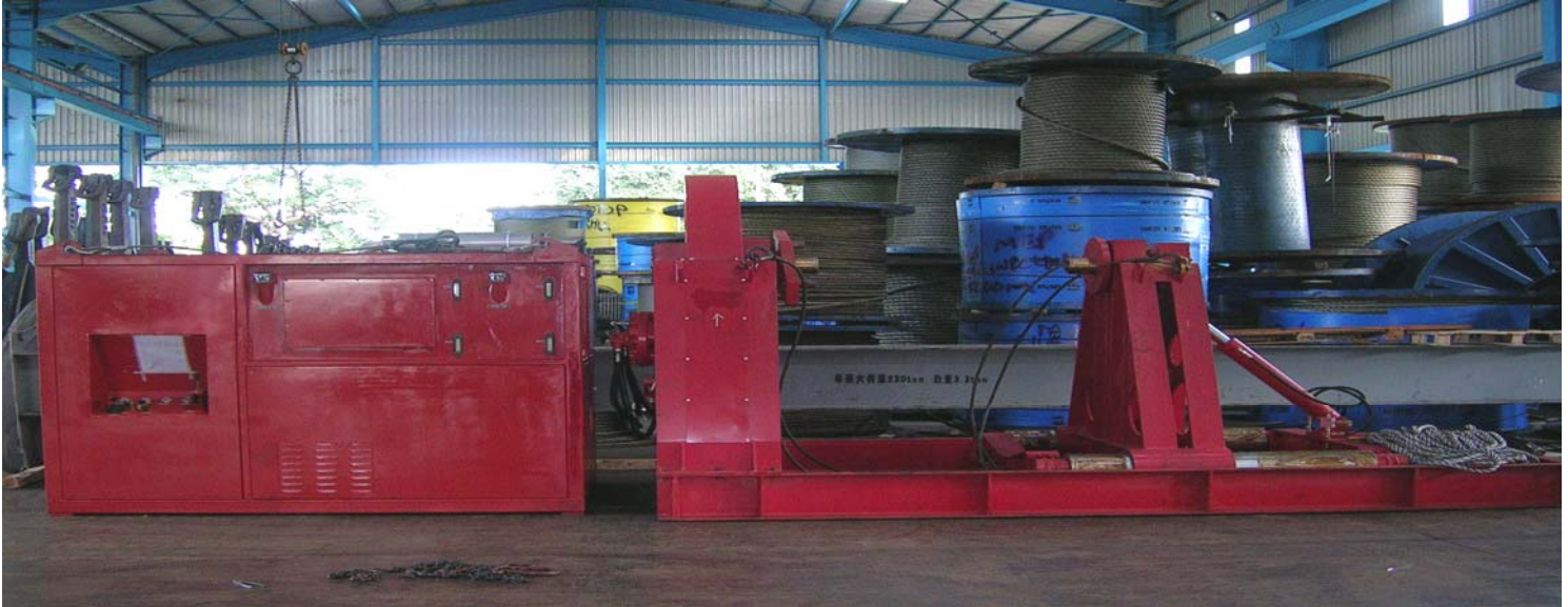
The “Oceanic 1” Spooling machine and diesel power pack
